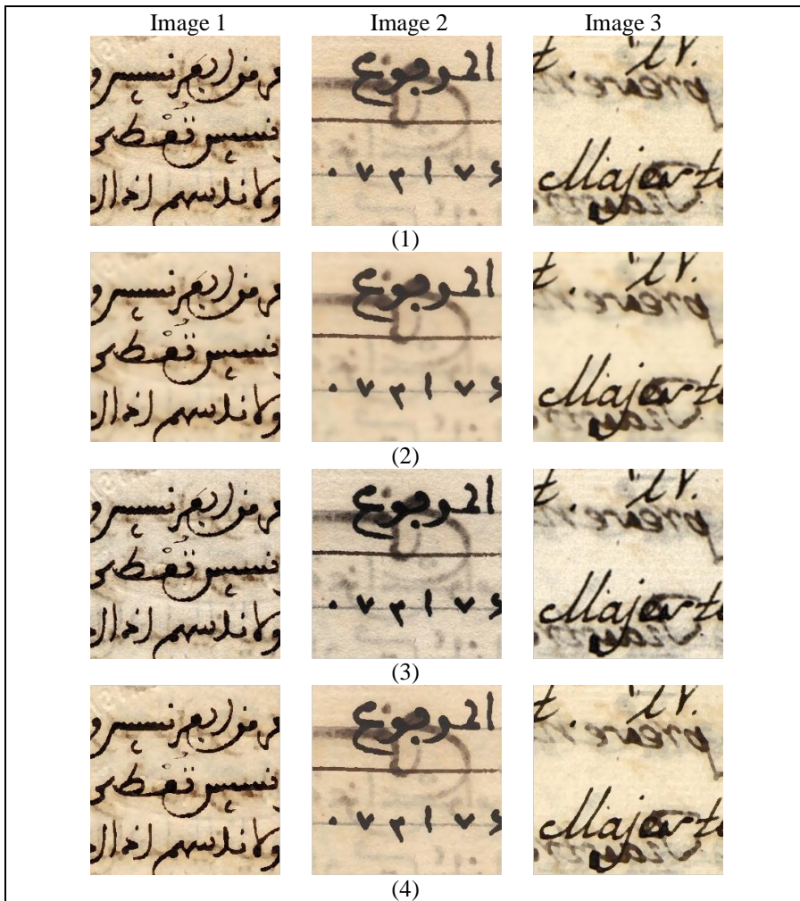
Figure. 2 : Comparison of denoising results obtained by the three approaches: (1) Original images, (2) Our approach, (3) Approach presented in [9], (4) Approach presented in [8]
